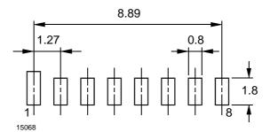
Figure 10. TFDT4500 Top View Package Note: Leads of the device should be at least 0.3 mm within the ends of the pads. Pad 1 is longer to designate Pin 1 connection to transceiver.
