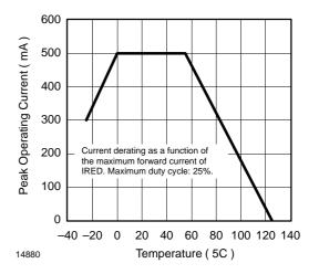
Figure 12. Current Derating Diagram
