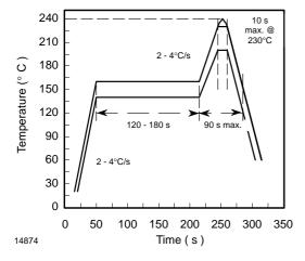
Figure 11. Recommended Solder Profile
