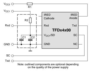
Figure 3. Recommended Application Circuit
